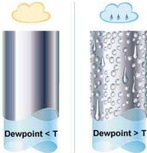
*A surface will not have condensation or ice formation on it, if the air in contact with it has a dewpoint lower than the surface temperature.*
