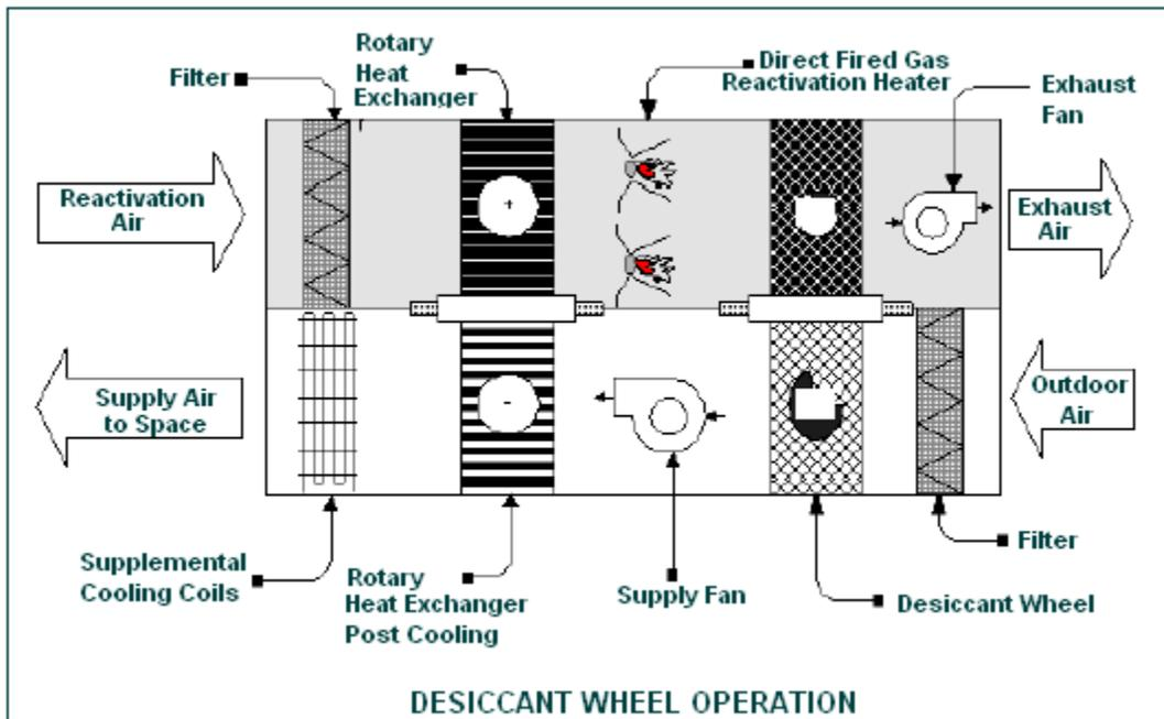
Desiccant systems often incorporate heat recovery equipment. If exhaust air is available, it can be used to cool the warm air (leaving the desiccant section) before it passes through the cooling coil. When there is no exhaust air, outside air can be used to cool this warm air, and the heated outside air can be used to reactivate the desiccant.
