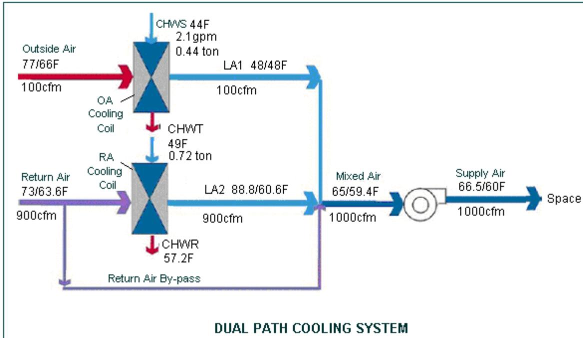
In chilled water dual-path systems, the outdoor air (OA) coil can use cold chilled water at 40°F to 42°F for latent cooling, while the return air (RA) coil can use warmer chilled water at
