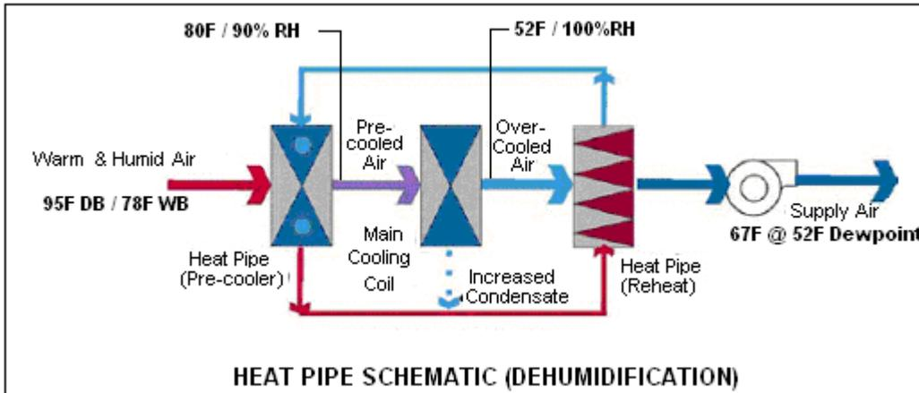
Heat pipe performance depends on the temperature difference between the cooling and the reheat coil banks. As outdoor air temperature decreases, the heat transfer across the heat pipe also is reduced so that eventually little or no reheat is available. Temperatures leaving the air conditioner with heat pipe added may vary significantly as the heat load changes.
