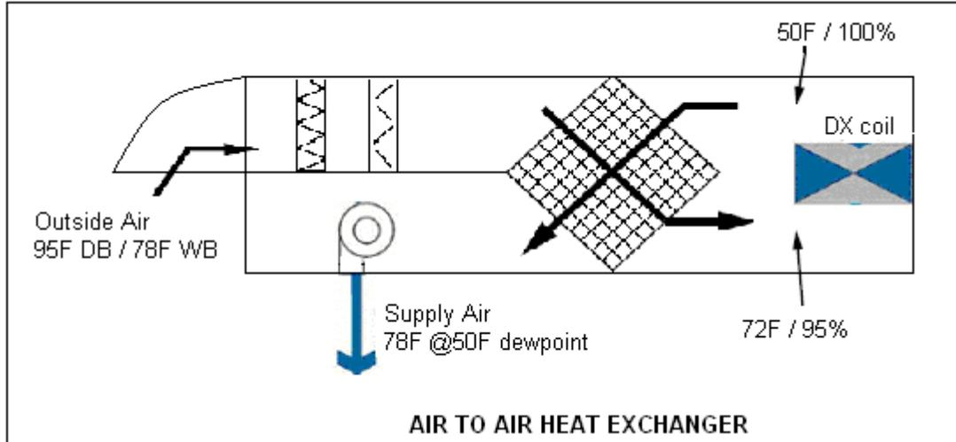
The efficiency of the heat exchanger is a function of the size and spacing of the aluminum fins and the temperature difference. As with the heat pipe, and for the same reasons, the amount of reheat and therefore the leaving air temperatures can vary significantly.
