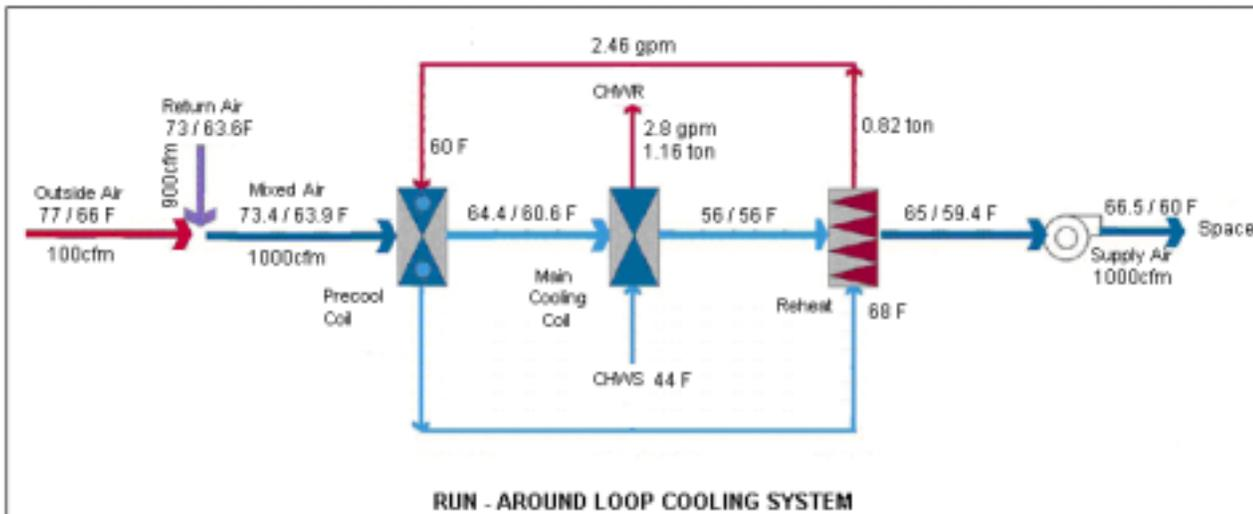
The heat recovery effectiveness of the run-around loop is defined as the ratio of the actual heat transfer to the maximum possible heat transfer between the air streams. This is equivalent to the ratio of the difference between the mixed air temperature and the air temperature off the precool coil to the difference between the
